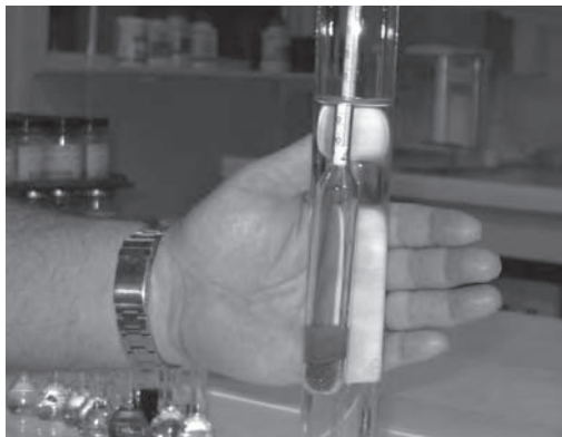
Figure 6.4 Salometer for assessing salt levels in processing brines.
