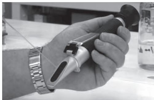
Figure 6.3 Salt refractometer for assessing salt levels in processing brines. One to two drops of brine are placed on the surface of the prism, and the cover plate lowered to produce a thin film of brine. The salt concentration is then determined by looking through the eyepiece.
